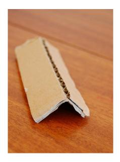
before folding. Notice the upper liner and the flutes have had to split in order for the fold to happen. This means the fold is only as strong as that bottom liner layer i.e. much weaker than if you'd folded it parallel to the flutes, as we did earlier.
