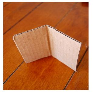
Suppose you needed to fold in the perpendicular direction. With very thick corrugated cardboard, you might not even be able to bend it in this orientation. So you'd score
